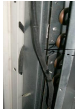
T4 sensor is worn out and connected with sheet metal
