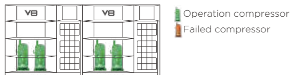
Intelligent load-bearing between units during normal operation
