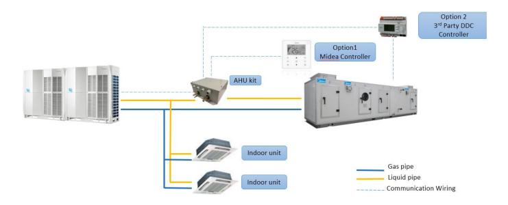
The system is composed by largely indoor and outdoor parts. Outdoor part is Midea VRF outdoor unit. Indoor part includes other brand direct expansion type AHU (Local supply) or Midea brand direct expansion type AHU and Midea DX AHU control box. AHU control box forms the connection between Midea VRF outdoor unit and other brand or Midea brand direct expansion type AHU.
