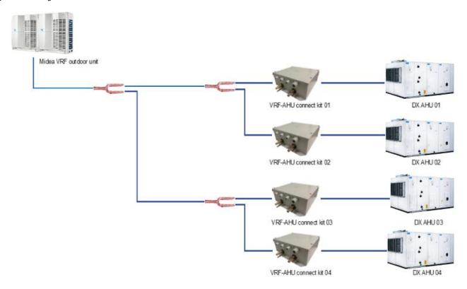
**Notes:** The example is just for application illustration. Only the liquid pipe connection is shown.
