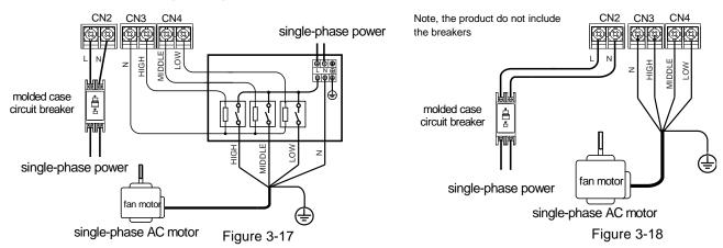
If wiring as shown in Figure 3-18, the maximum current of the fan motor must not exceed the value shown in Table 12-10.5.
