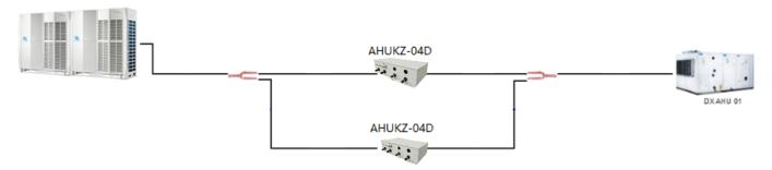
Notes: The example is just for application illustration. Only the liquid pipe connection is shown
