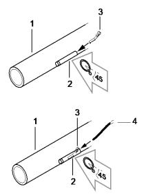
3. Apply insulation materials and secure with cable ties.
