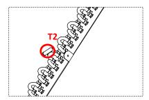
3. T2B is an AHU evaporator outlet sensor; it should be installed at the outlet pipe of the evaporator.
