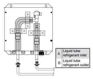
2. For the kit with two or three EEVs, the EEV inlet and outlet need to be connected through branch joints separately.
