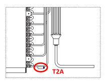
2. T2 is an AHU evaporator intermediate temperature sensor; it should be installed at the intermediate pipe of the evaporator;
