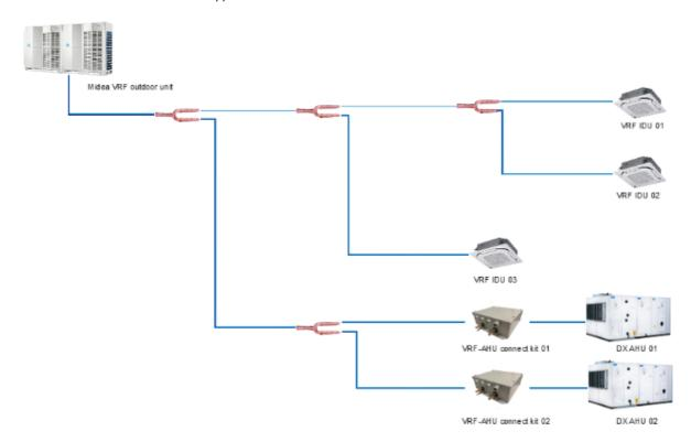
Notes: The example is just for application illustration. Only the liquid pipe connection is shown
